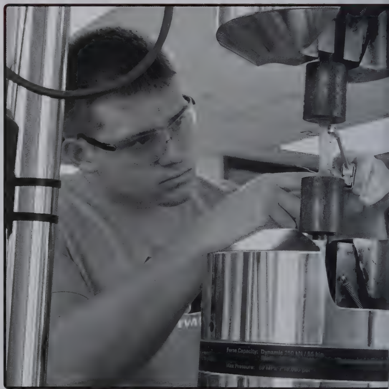
With calculated precision, junior Ethan Welch uses an extensometer to steady the polymer rod. Welch hopes that the rod will break in the middle when the machine pulls at each end. | Taylor Williams
